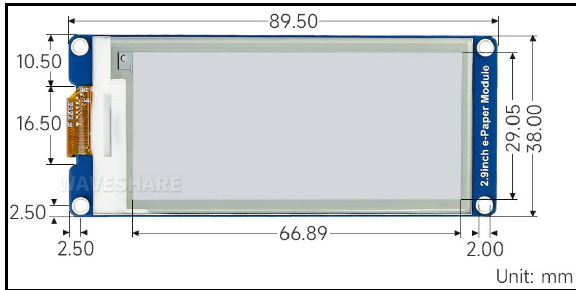
Fig. 27 Dimensions of the Waveshare E-INK display module
